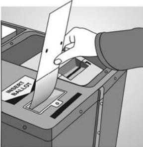
A **Precinct Ballot Reader (PBR)** that sits on top of the Ballot Box. The PBR checks ballots for Overvotes (more selections than a contest allows) and completely Blank Ballots. It notifies voters of either error by printing a Ballot Alert Notification Slip, thus providing a second chance to correct the ballot.
